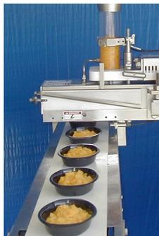
To ensure easy positioning on the line, the filling head is mounted on the product in-feed conveyor. The head section features:
