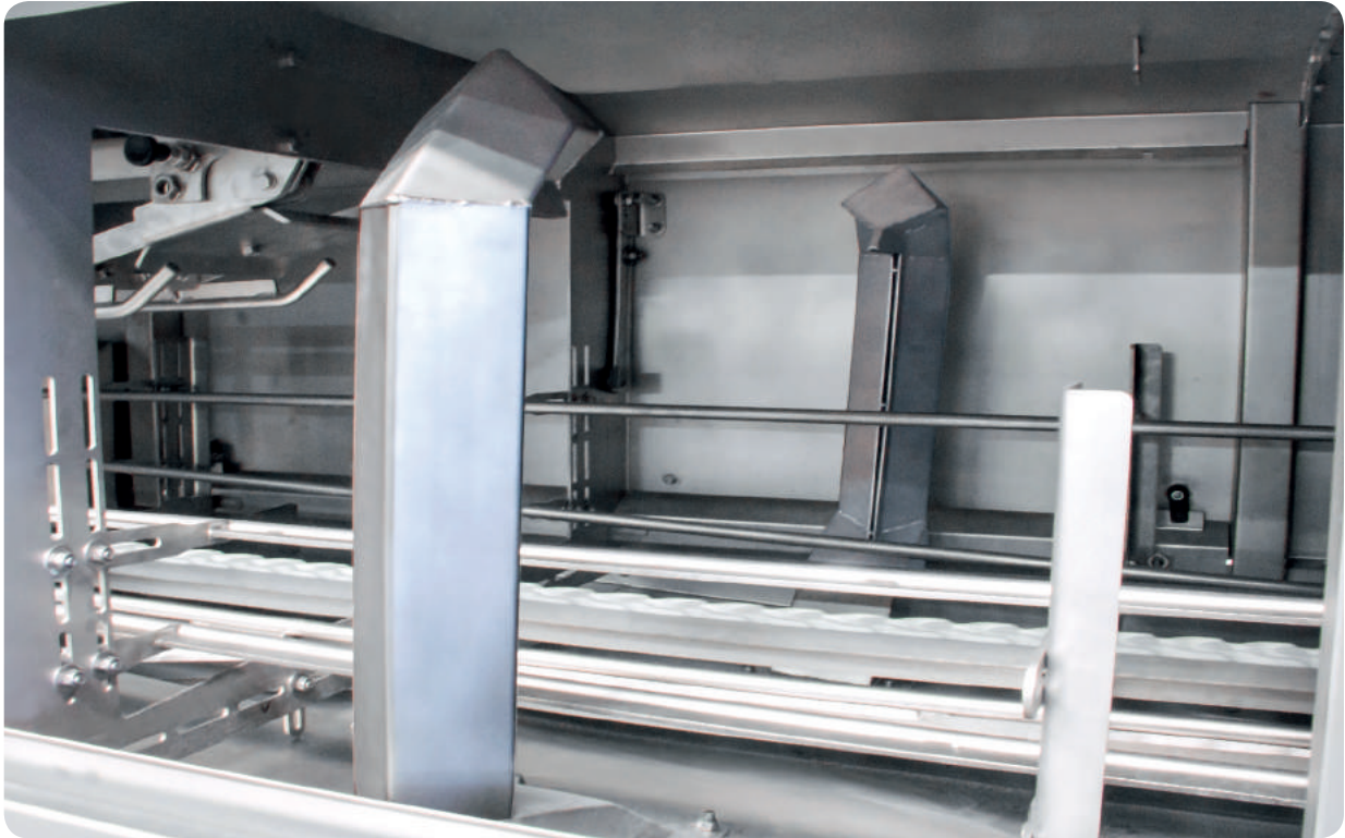
The inner workings of the EAB-1-ST, the air blades 'cut' the residual water from the crate.
