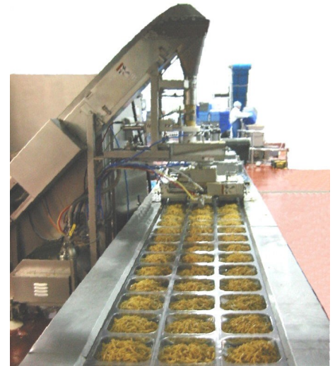
Six-position distribution system filling Chinese noodles at speeds up to 72 cpm
