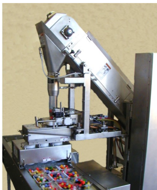
Three-position distribution system with MPFSC-120-01 filling machine
