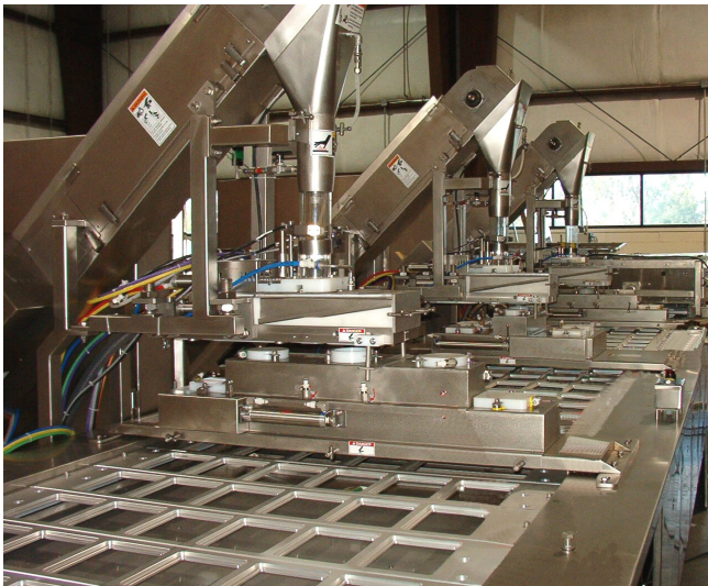
Three each, four-position distribution systems at speeds up to 252 cartons per minute (21 cycles x 12 containers)
